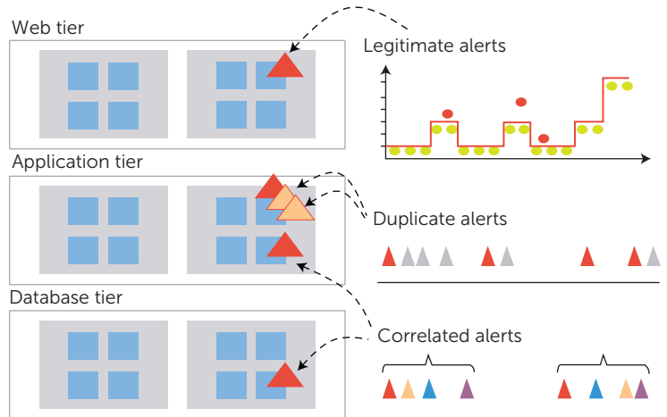
FIGURE 7. Enterprises can use analytics to identify types of alerts, allowing them to choose which alerts to act on.
