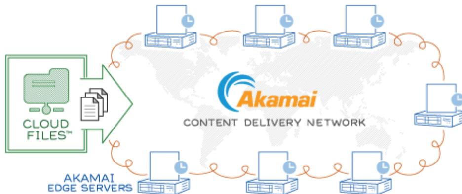
Fig. 4. Architecture of Rackspace Cloud Files
