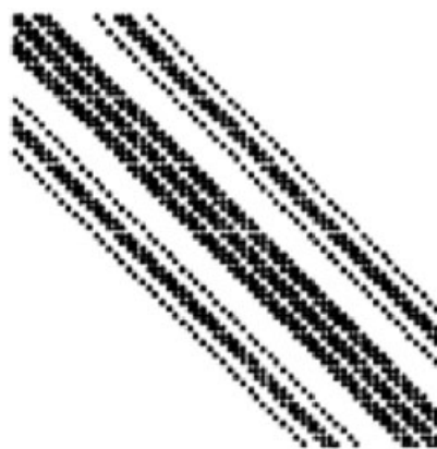
Figure 3. The sparse pattern of the matrix associated with 4 \times 4 \times 4 grid points.
