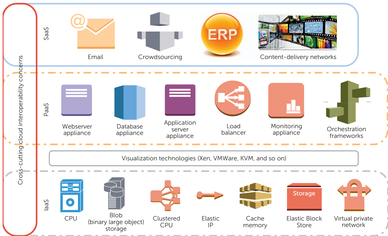
FIGURE 1. Layered architecture of cloud computing (adapted from earlier work. 2 )
